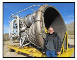
ever flown. **Five** of these engines clustered together to power the first stage of the Saturn V rocket, which carried men to the moon. One of these engines is a height of 18' 3", diameter of 12', and weight of 18,616 lbs.
