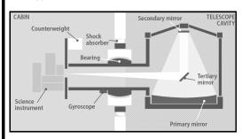
**SOFIA Airborne Telescope Diameter -** Like most modern research telescopes, the SOFIA telescope uses a mirror to concentrate and focus the incoming light. SOFIA's telescope is usually referred to as a 2.5-meter meter telescope, rather than 2.7 meters, because the optical design requires that only about 90% of the mirror's reflecting surface (called the "effective diameter") can be used at any one time.
