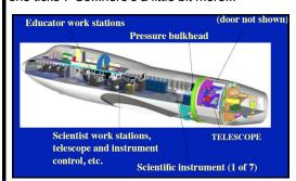
**SOFIA Airborne Telescope Stabilization** - How do you keep a 19 ton, 100" diameter telescope, which is mounted in the rear fuselage of a modified Boeing 747SP aircraft stable while flying at 40,000 feet? First, isolate the telescope from the airplane by mounting it on a spherical pressurized oil bearing. Second, direct the wind away from the telescope by shaping the side of the airplane so as to deflect it. Third, stabilize the telescope against sudden motion by spinning three gyroscopes.
