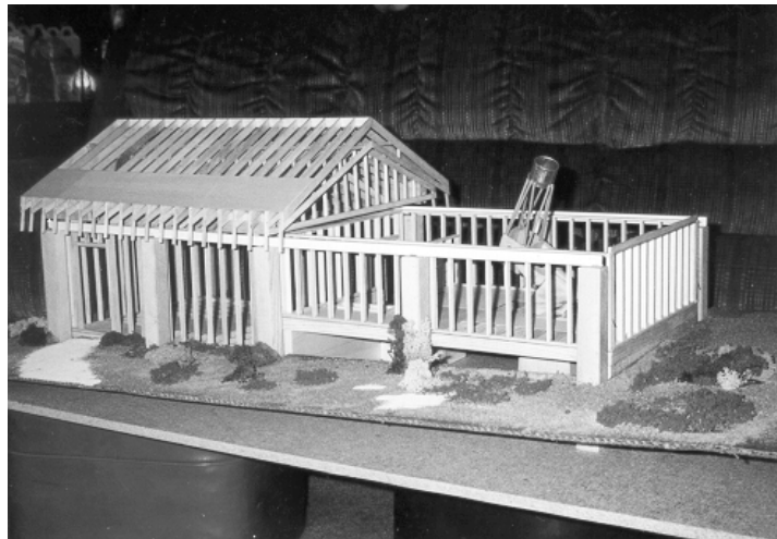
The same view of the observatory with the roof retracted to the north to expose the 16' x 24' viewing area and Panarusky Telescope.
