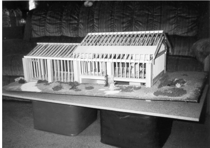
A look at the 1/16 scale concept model of the roll-off roof observatory as it would appear when closed up. The walls remain open to allow for viewing the construction details
