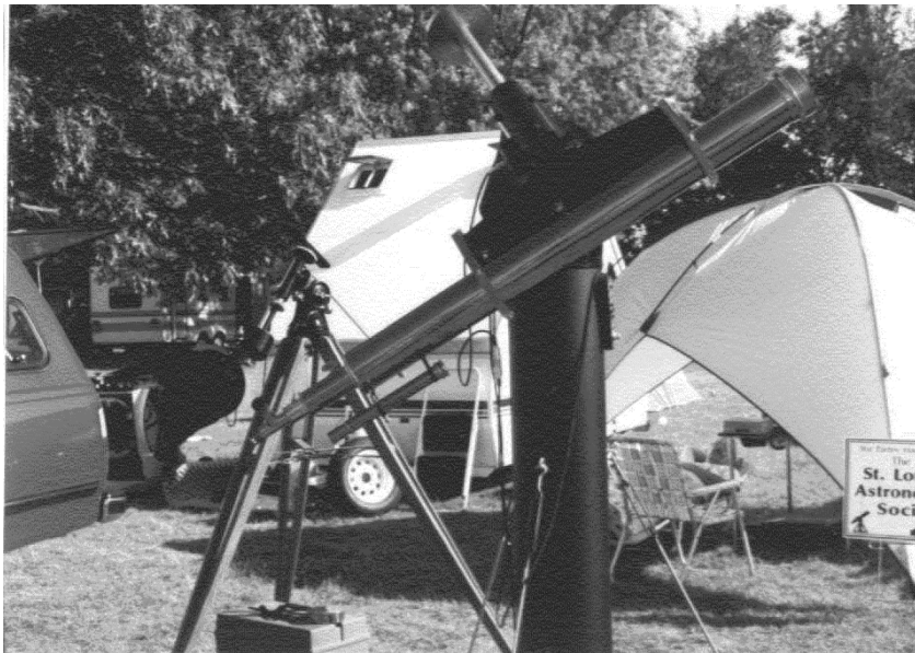
A refurbished Alvan Clark refractor mounted on an Astrophysics mounting. It is set up with a special device for viewing the sun called a Herschel Wedge.
