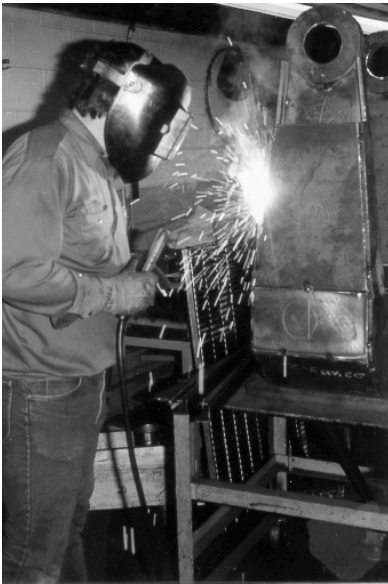
"Happ" DeWitt welding 1/2 " steel plates together to form the Fork.
