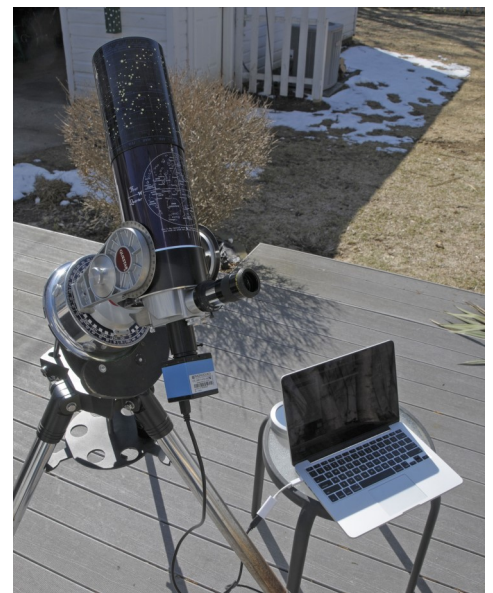
The author's 3.5 Questar is set up for photography, with the camera on the axial port, a par-focal eyepiece on the viewing port, and a laptop with software to capture a rapid-fire series of images.
