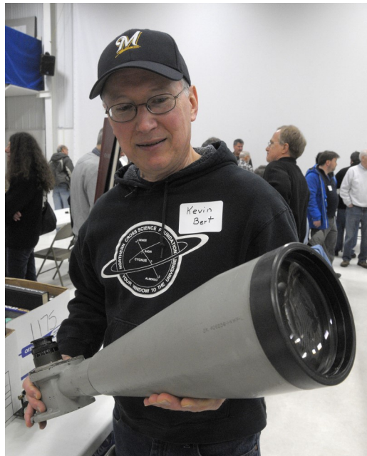
Kevin Bert holds the military-grade Moonwatch Apogee scope, which he'll use as a rich-field refractor.
