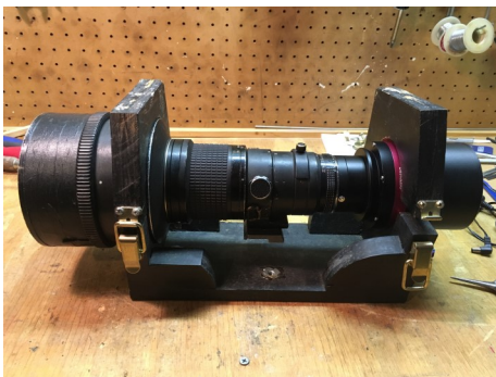
The Nikon lens and astro camera in the workshop, being refitted into custom cradle I made years ago for a film camera and lens.
