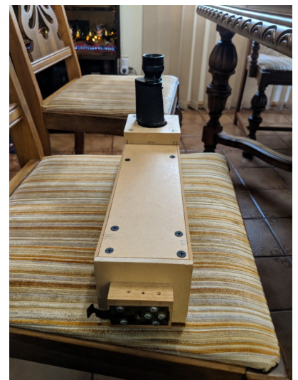
Jason's spectroscope. Notice the 1/2 binocular (sawed off) used to image the spectrum produced.
