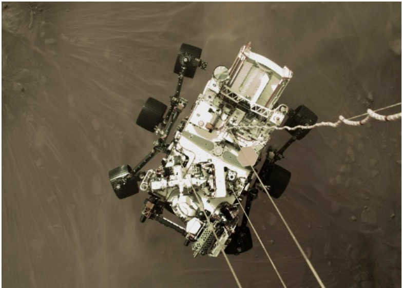
Clockwise from above: Just seconds from touchdown, the rover is suspended from the descent stage's sky crane as dust kicks up from the rocket exhaust.
