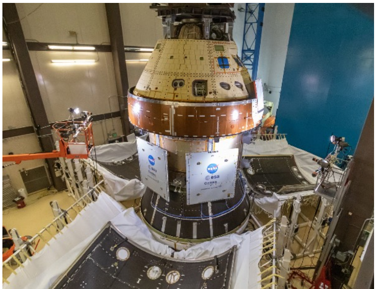
The Lockheed Martin Orion spacecraft undergoes a jettison test of the service module fairings on June 1, 2020 at a Lockheed facility near Denver. This and other Orion photos can be seen at Lockheed Martin's Flickr website .
