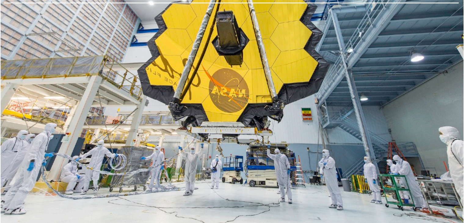
NASA technicians examine the fully-deployed primary mirror of NASA's James Webb Space Telescope during testing at the Goddard Space Flight Center in Greenbelt, Maryland in 2017. The 18-segmented gold mirror is designed to capture infrared light from the first galaxies that formed in the early universe. NASA photo
