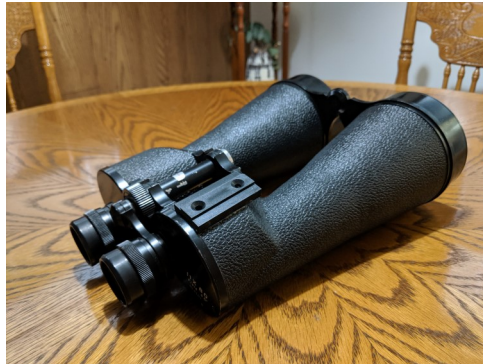
Mounting bracket epoxied to binoculars.
