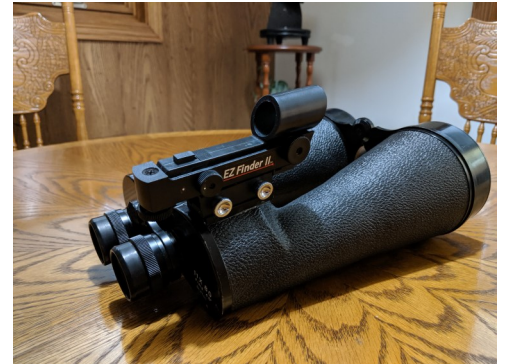
Red Dot Pointer mounted to bracket.
